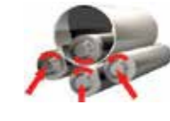
HRB-4R RECTILINEAR ROLLS SYSTEM Top Roll: Ø 460-Ø760 mm Drive: All Rolls
